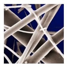
Figure 1 Electron microscope image of fibre media air filters
