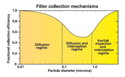
*Figure 2 Fractional collection efficiency versus particle size for a mechanical filter.*
