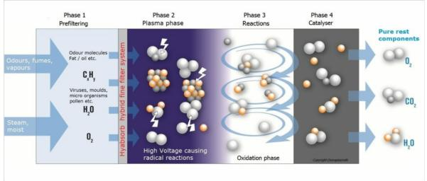
Figure 7 Plasma air filtering process (source: http://www.domaplasma.com)
