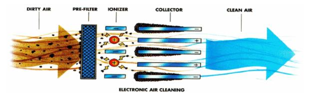
*Figure 3 ESP operational diagram (source: http://www.airscrubbersinc.com)*
