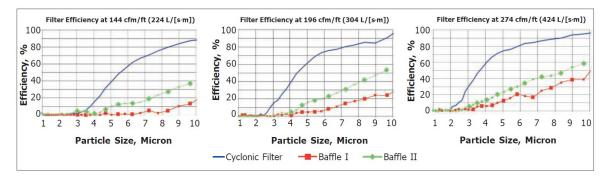
*Figure 6 Grease filter efficiency as function of particle size for three exhaust airflows (Livchak et al., 2003)*
